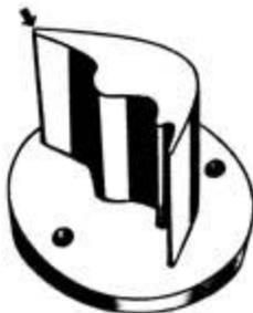
Conventional Steel—Cracking and fracturing at the tip of the long, thin shape, shortened life.
