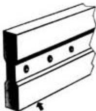
Conventional Steel—In the first stages of use, chipping of blade edge occurred marking the beginning of blade wear.
