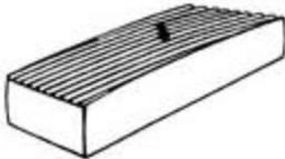
Conventional Steel—Chipping and local seizing of threads, required early regrinding.
