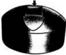
Conventional Steel—Chipping of the cutting-edge and insufficient base hardness of the die led to termination of life.
